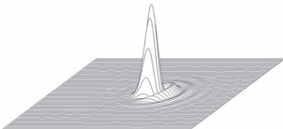
Figure 1. Uncorrected coma leads to irregularly shaped focus spots or a change in magnification with field angle. This illustration of the point-spread function of a lens with coma shows clearly non-symmetric wavefront distortion.
